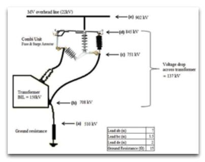
Figure 8: Voltage drop calculations of Combi configuration
