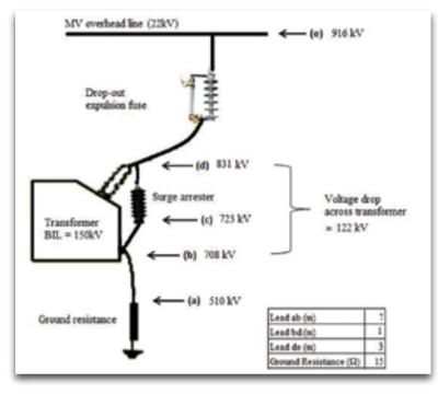
Figure 7: Voltage drop calculations of standard configuration
