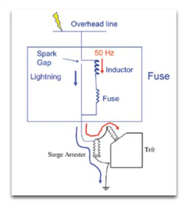
Figure 2: Circuit configuration using a Lightning Proof Fuse.
