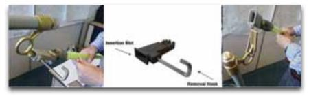
Figure 10: The insertion tool to replace drop out surge arresters & fuses
