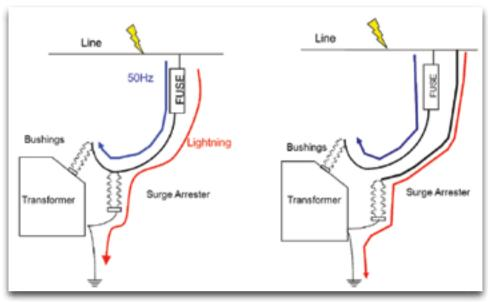
Figure 5 (A) Standard pole mounted transformer configuration and (B) Combi unit configuration
