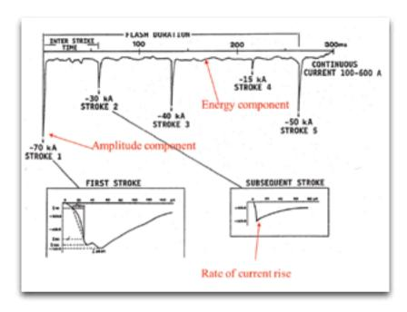
Figure 1: Three basic components found in a lightning flash [1]
