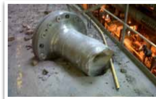
Figure 2: A Section of the Main Shaft Approximately 360mm Diameter
