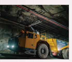
Boliden, Epiroc, and ABB have passed a new technology milestone by successfully deploying the first fully battery-electric trolley truck system on an 800-meter-long underground mine test track in Sweden, with a 13 percent incline. This means the mining industry is a step closer to realising the all-electric mine of the future, with sustainable, productive operations and improved working conditions.
