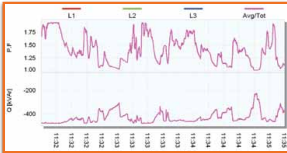
Figure 2: Capacitive Power Factor at PCC with Utility
