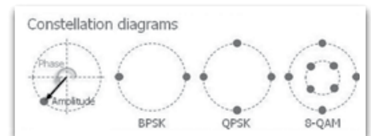
Figure 1: M-PSK and M-QAM modulation formats
