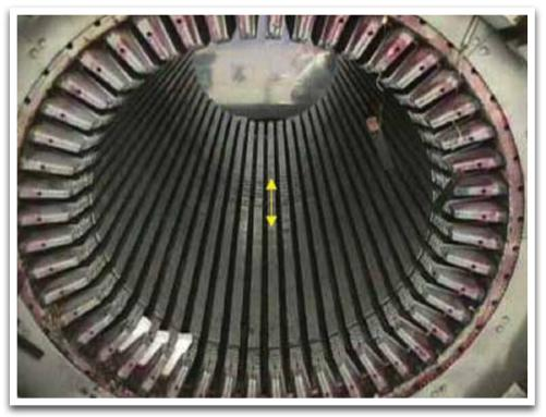
Fig 22: Photo of the Core Showing the Vented Section in the Middle.
