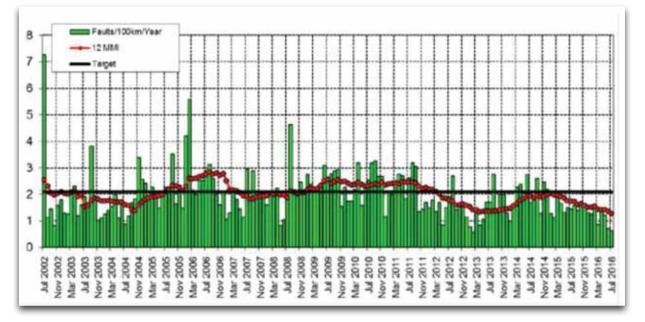
Figure 10: Eskom Transmission 400KV Faults / 100km
