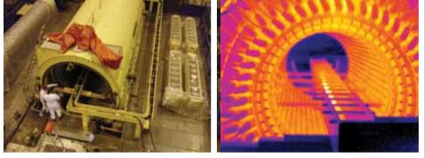
Fig 6: Rated Flux Test Setup and View Through Thermal Camera on a 600 MW stator
