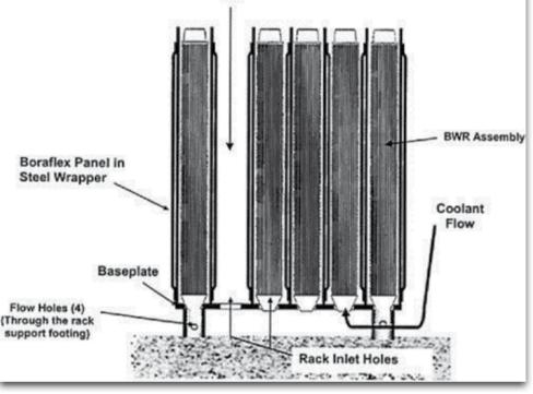
*Fig. 1: Boraflex as an absorber insert [9]*
