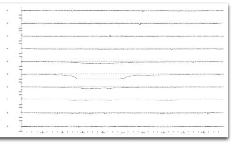
Fig 7: EL CID Overview Results for slots 35 – 45
