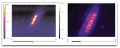
Fig 9: View of slot 40 through Thermal Imaging Camera Before and After a Repair Attempt
