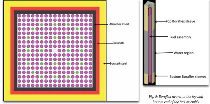
Fig. 2: Neutron absorber insert inside the fuel assembly flask
