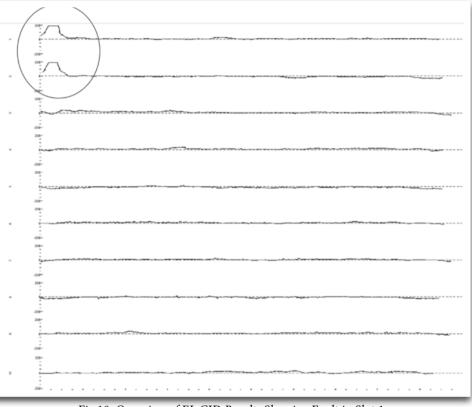
Fig 10: Overview of EL CID Results Showing Fault in Slot 1
