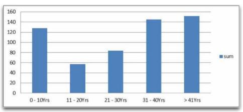
Figure 2: Eskom Transmission transformer age distribution
