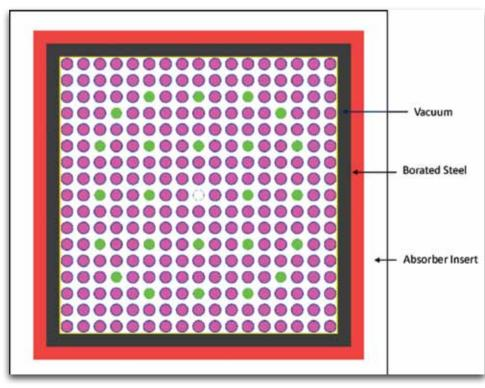
Fig. 3: Neutron absorber insert outside the fuel assembly flask
