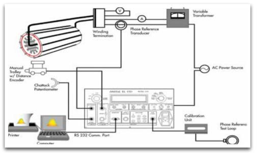
Fig 2: Sketch from EL CID Manual showing EL CID Test Setup
