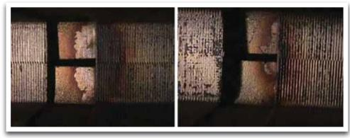
*Fig 23: Close up View of the Hotspots Between the Vent Duct Spacer and the Core Laminations.*
