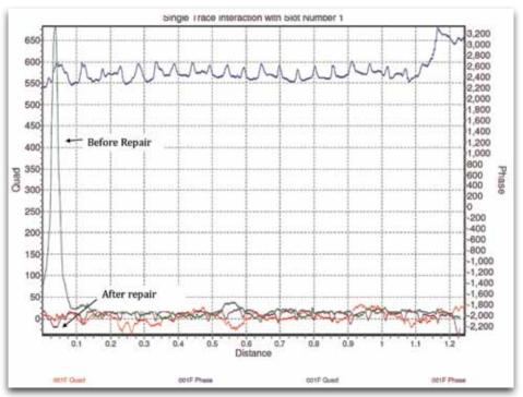
*Fig* 14: Close Up View Showing the Before Reading in slot 1 (green trace) and After (red trace).
