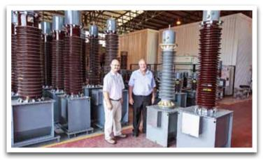
Nick de Beer (right), Product Manager, Instrument Transformers, and Etienne Venter, Design Engineer, Voltage Transformers, of ACTOM High Voltage Equipment stand next to a compact 132kV voltage transformer, which is substantially smaller than the conventional units around it, as the picture shows.
