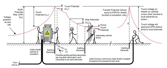
Figure 2: In the event of an earth fault current or large neutral current (in the event of a severe phase unbalance) injected into the neutral earthing system, it will give rise to a ground potential rise, commonly referred to as GPR. This GPR will transfer to the vicinity through the conductivity of the soil and also via conducting parts of the electrical system
