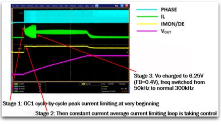
Figure 5. Bench Waveforms of SC Charging
