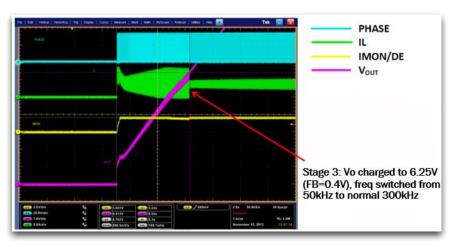
Figure 7. Bench Waveforms of SC Charging
