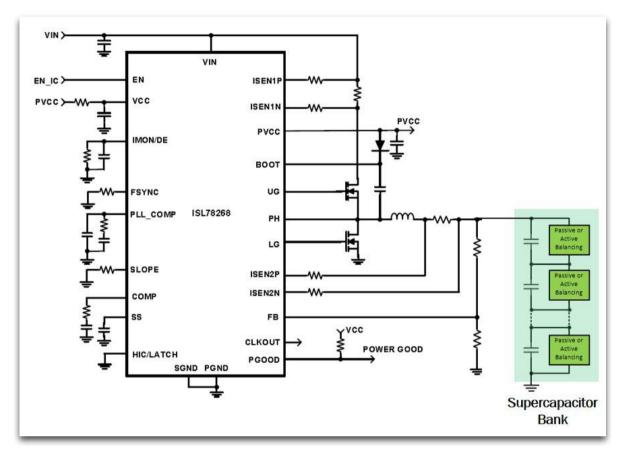
Figure 3. Simplified Schematic of a Sync Buck Regulator Achieving CICV SC Charging Control
