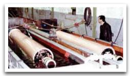
was done at a shipbuilder in Deggendorf, on the river Donau, in the south-east of Germany. Two reference edges, 4 m apart, were machined at the rear of each chamber. When Johan controlled this distance with his 5 m tape measure, which he used to check all dimensions, it agreed to within 0.1 mm. Johan still has this tape measure, which helped to ensure that the parts of the SSC fitted together, after timely correction of some errors indicated by it.
