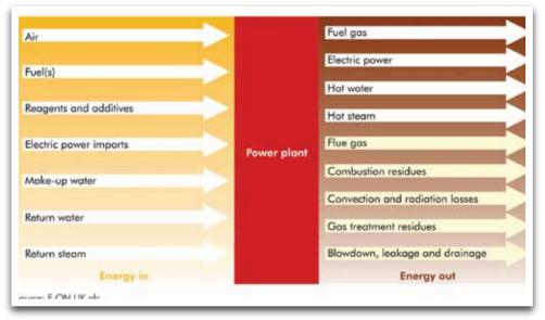
*Figure 9: Example of a process boundary showing energy in-flows and out-flows for a power plant*
