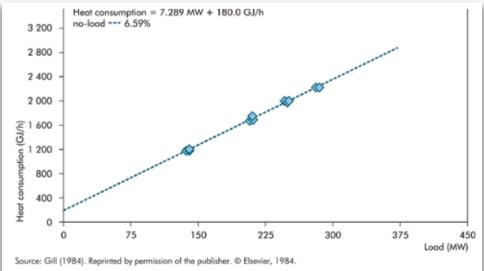
*Figure 1: Typical relationship between steam turbine heat consumption and operating load*
