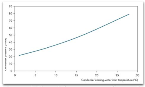
*Figure 4: example of the impact of cooling-water temperature on condenser pressure for constant unit load*
