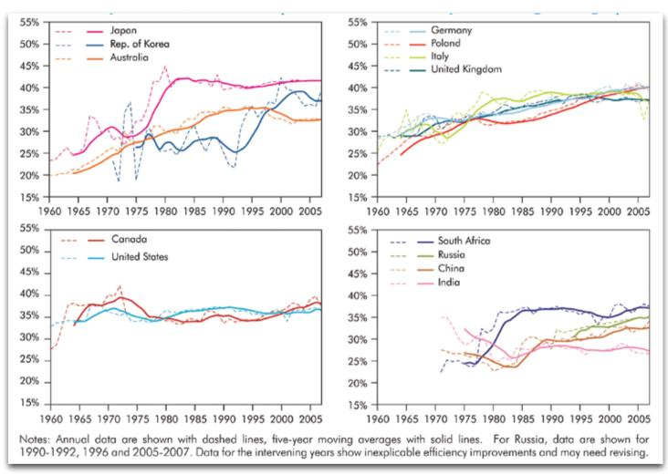
*Fig 10, 11, 12 and 13: Evolution of coal-fired heat and power plant efficiency in selected countries (annual data and five-year moving averages)*
