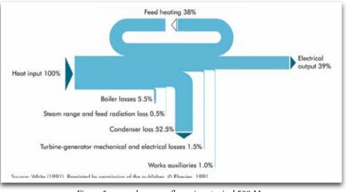
*Figure 3: example energy flows in a typical 500 Mw subcritical pulverised coal-fired boiler*
