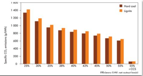
Figure 8: example of relationship between Co<sub>2</sub> emissions and net plant efficiency (with and without CCS)
