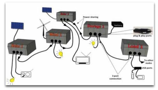
Figure 2: A Picogrid with five nodes (each with a three-port connection)
