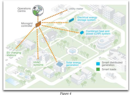
A typical microgrid for a large university campus, showing microgrid controller and distributed energy assets.
