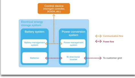
Figure 5 Energy storage system components
