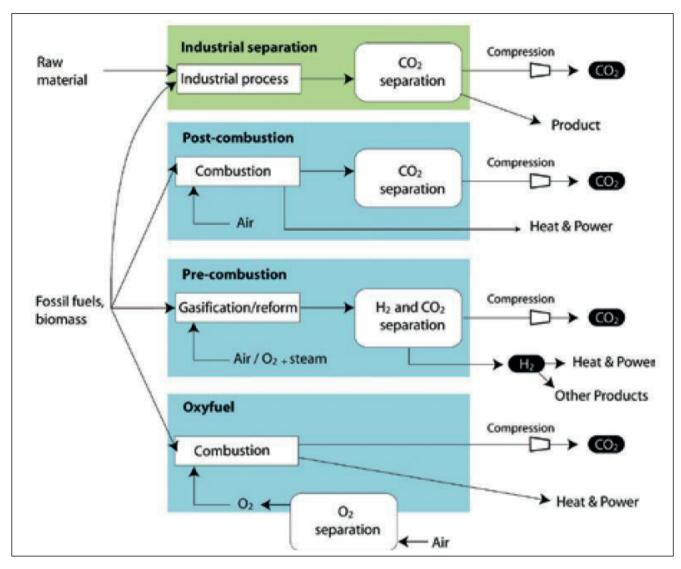
Figure 2: Schematic presentation of carbon capture processes (courtesy CO₂CRC)
