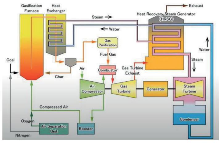
Figure 4: Typical IGCC plant process
