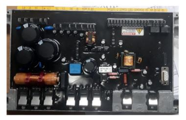
Fig. 5: Automatic Voltage Regulator
