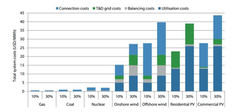
Figure 7 Grid-level system costs of selected generation technologies [5]
