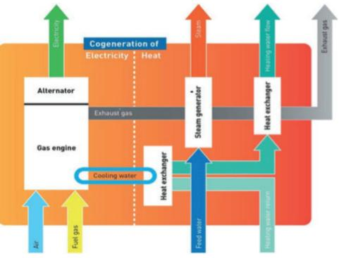
Fig. 2: Typical Flow Diagram (Courtesy of MWM)
