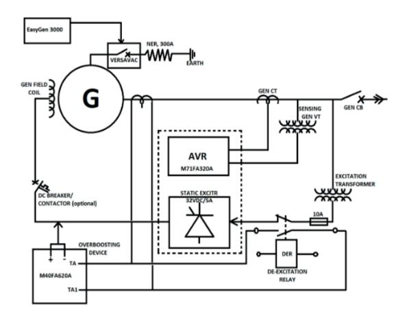
Fig 3: Application Setup of the Co-Generator Alternator & Excitation System
