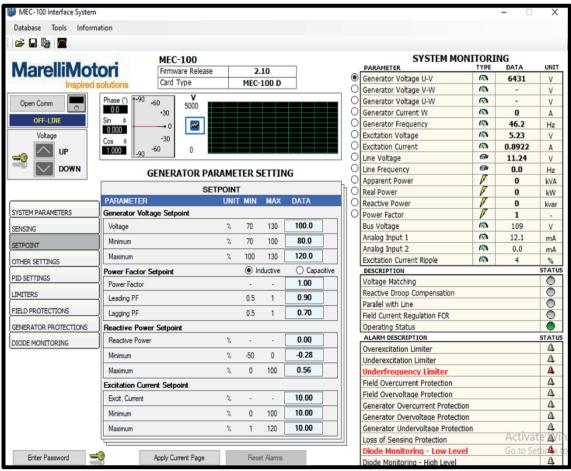
Fig. 8: Faulty Excitation System indicating "Rotating Diode Monitoring-Low Level.
