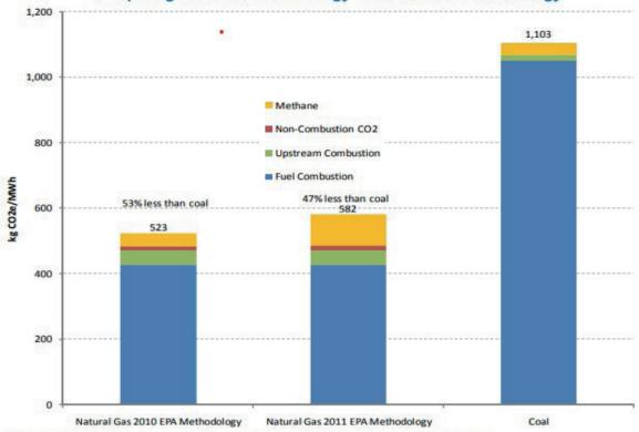
Figure 4: Average Life-cycle GHG Emissions for Coal and Gas Electricity Generation (Source DBCCA [7])
