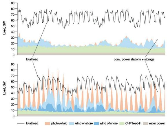
Figure 3: Effect of Renewable Generation Penetration (Source IEA)
