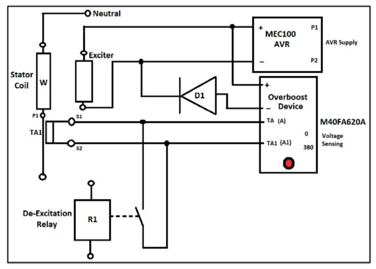
Fig. 7: Typical Schematic of the Excitation System
