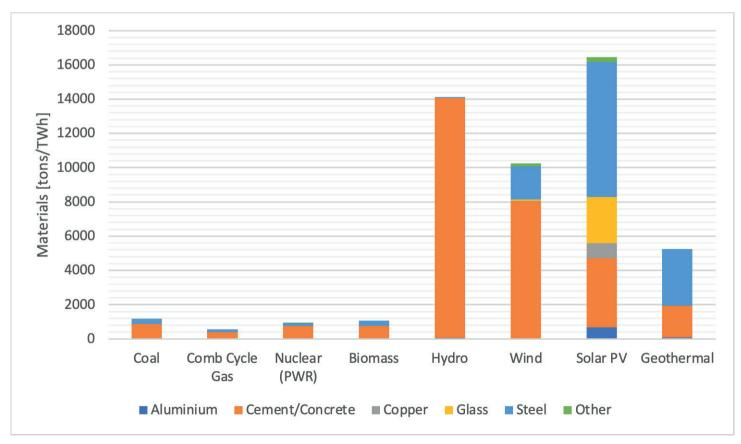
Figure 8: Material Input in tons per Unit of Service [TWh] adapted from DOE Report [16]
