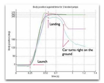
*Fig. 4. Graph of yaw position against time for three successful jumps (in colour) and the simulated controller response (black). It should be noted that the robot's steering was not controlled, and it often turned right after landing.*
