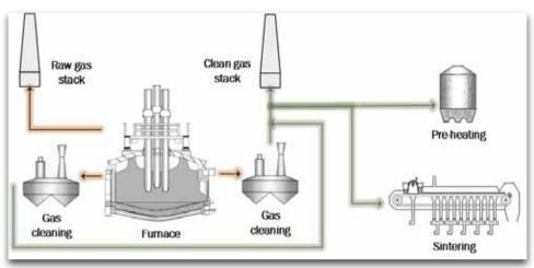
Fig. 1 Ferrochrome smelter off-gas flow diagram.
