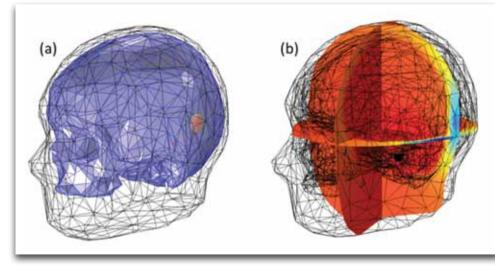
Figure 2. (a) Visual representation of the finite element mesh of the full head model showing the external return electrodes in red. (b) Predicted potential fields as a result of intracochlear stimulation on two planes through the model. The cochlea can be seen as a dark area behind the vertical plane and below the horizontal plane.
