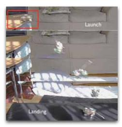
Fig. 3. An actuated jump sequence, which resulted in a successful landing. Five frames are shown, with the robot at launch, 90, 180, 270 and 360 degrees.
