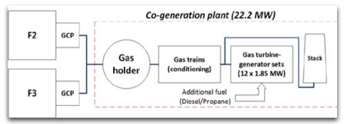
Fig. 5: Basic layout of a possible gas turbine co-generation plant at the FeCr smelter
