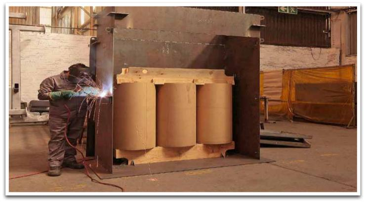
A welder works on a full-scale model that was made to facilitate achieving the optimum design for the new wind farm transformers.
