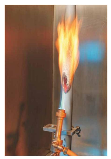
Helukabel fire testing of cables
