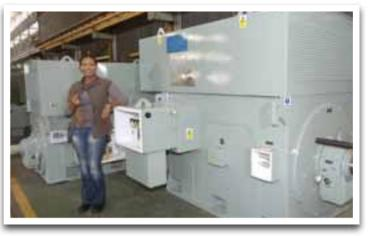
Mpho Motloung, a Contracts Engineer for ACTOM Electrical Machines, checks over some of the motors produced for Eskom's power stations.
