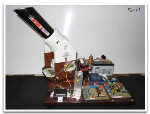
coil, as well as a piston, with a piece of aluminum attached to the base. As soon as the thyristor was switched open, the current pulse in the coil would cause eddy currents in the aluminum plate, which lead to opposing magnetic forces, launching the piston forward to strike the projectile.
