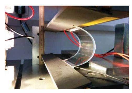
A flexible organic solar cell from TREASORES project undergoing mechanical testing: the cell is repeatedly flexed to a 25 mm radius whilst monitoring its performance. Such cells have shown lifetimes in excess of 4000 hours. Credit: National Physical Laboratory (NPL), England
