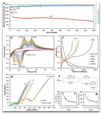
Figure 4 | (a) Cycling data of nano-Si@C anodes with selected C-rates (C 5 4Ag<sup>21</sup>). (b) CV plot of the first 13 cycles using a scan rate of 0.02 mVs<sup>21</sup>. (c) Charge-discharge curves for selected cycles. (d) EIS curves for selected cycles showing both experimental and fitted-model data. (e)Equivalent circuit of nano-Si@C electrodes used to produce fitted-model data. Extracted resistance values from the EIS curves for (f) charge transfer resistance and (g) SEI 1 INT resistance.
