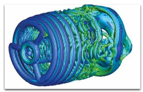
This large eddy simulation shows air going through a dual-rotor wind turbine. (The three lines at the front are the blades of the main rotor; the secondary rotor is embedded in the ring near the centre.) By tailoring the rotation and turbulence behind the turbine, Iowa State engineers say the dual rotors can boost the recharge of wind loads. And that can improve the energy harvest of wind farms. Credit: Anupam Sharma
