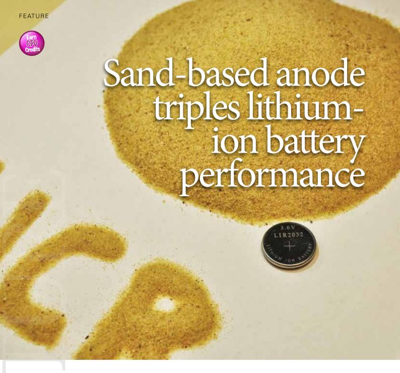
Porous nano-silicon has been synthesized via a highly scalable heat scavenger-assisted magnesiothermic reduction of beach sand. This environmentally benign, highly abundant, and low cost SiO<sub>2</sub> source allows for production of nano-silicon at the industry level with excellent electrochemical performance as an anode material for Li-ion batteries
