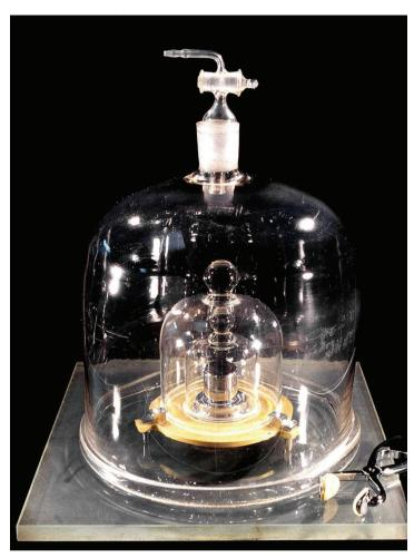
International Prototype of the Kilogram kept in three bell jars in an underground vault of the BIPM at Sèvres.
