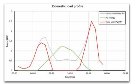
*Figure 8: Typical load profile for a residential house with a 1200 W grid-tied photovoltaic system.*
