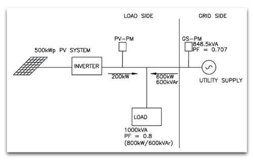
*Figure 1: Active and reactie power flow for a load with unity rated power factor grid-tied photovoltaic system.*
