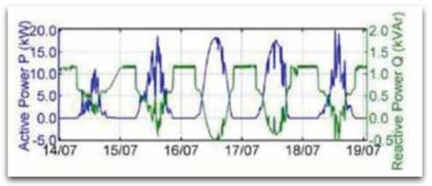
Figure 2: Real and reactive power flow measureents from a unity rated grid-tied inverter [3].
