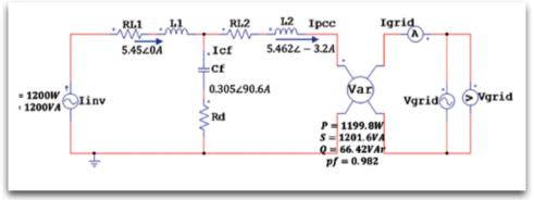
*Figure 6: Calculated reactive power and currents caused by the inverter filter, when the photovoltaic system is producing 1200 W at unity power factor.*
