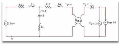
Figure 4: Equivaelnt circuit diagram for analysis of a grid tied inverter with LCL filter.
