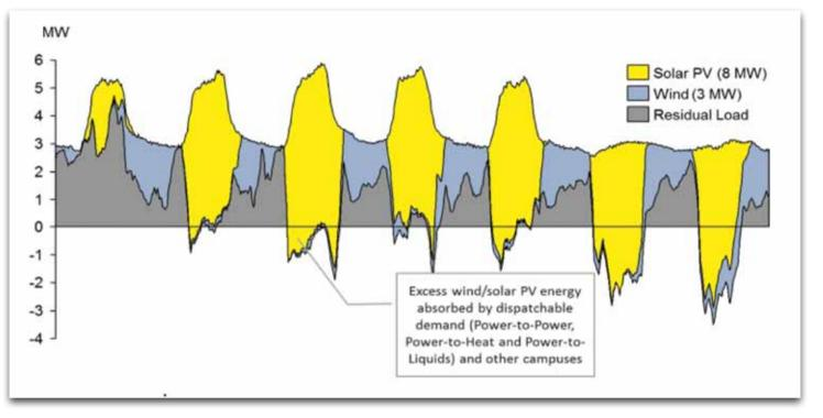
*Figure 7: Illustration of campus energy supply with a combination of renewable energy sources.*
