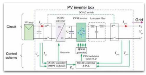
Figure 3: General components arrangement for a typicl grid connected inverter [6].
