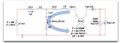
*Figure 5: Calculated reactive power and currents caused by the inverter filtr when the pv system is producing zero amps.*
