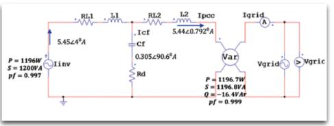
*Figure 7: Calculated reactive power and currents caused by the inverter filter, when the pv system is producing 1200 VA at 0.997 p.u. power factor.*
