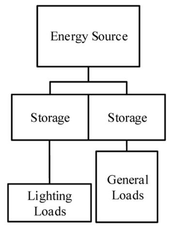
Figure 1: Nanogrid Configuration
