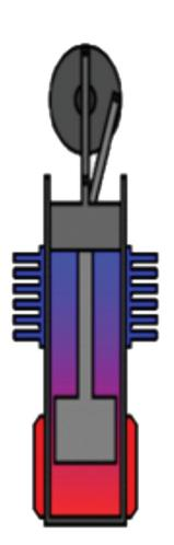
Beta type with one cylinder. The displacer piston does not make contact with the cylinder and requires no lubrication. The power strokes are provided by the cold piston. The renegerator function is provided by the displacer piston and cylinder walls.
