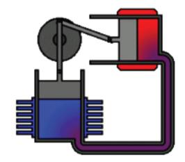
Alpha type with two cylinders. The pistons of the hot (red) cylinder and the cod (blue) cylinder are 90° out of phase on the crankshaft. The regenerator connecting the cylinders improves efficiency by cooling the gas as it moves to the cold cylinder and heating it as it returns to the hot cylinder.
