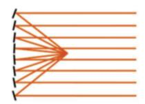
Parabolic trough reflector compared to linear Fresnel reflector.
