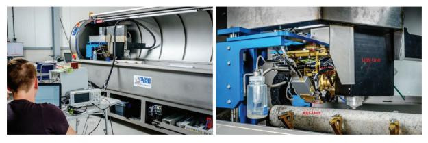
Figure 1: LIBS-XRF core scanner prototype
