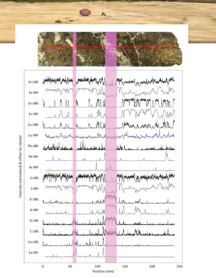
Figure 2: LIBS and XRF results of scanning a polymetallic sulphide ore sample. The pink bands indicate the position of quartz/calcite veins.
