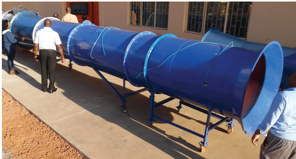
M&C Zambia test technicians conducting a test with the facility's newly installed mine ventilation fan test column.
