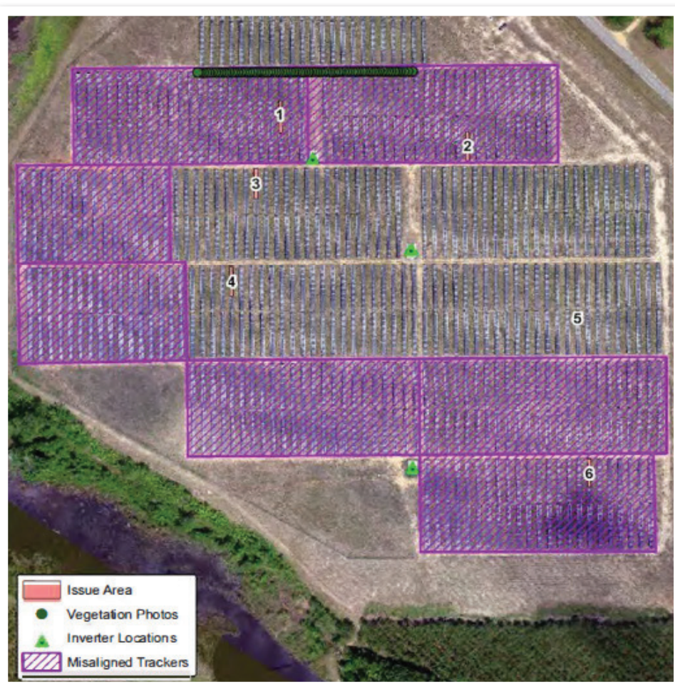
Fig 2 - Inspection Overview. Visual orthomosaic displaying key site features and issues identified. This image was created via georeferenced imagery collected by drone flyover and later stitched together into a single site overview.
