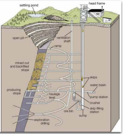
Figure 1: Cross-sectional view of underground mining operations
