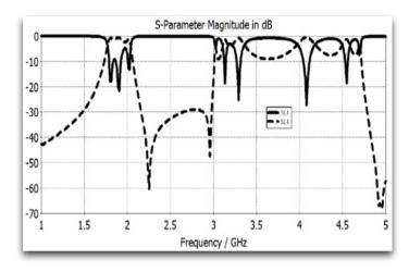
Figure 3: Output of three-polar band-pass filter
