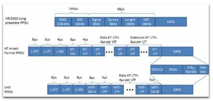
Figure 6: Example physical layer frame formats with 802.11b, n and ac. [source: EKAHU]
