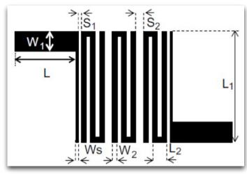
Figure 1: Two-dimensional design of three-polar band-pass filter
