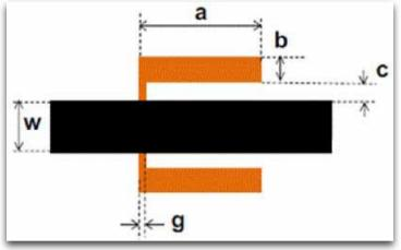
Figure 6: The structure of designed defected ground
