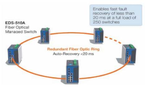
Figure 12: Example illustrating ring redundancy [source: 9]
