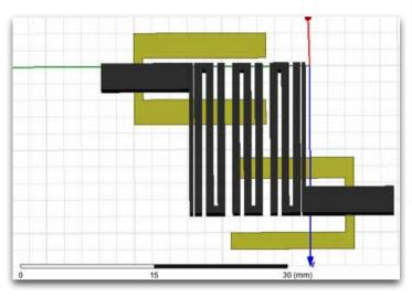
*Figure 4: Three-polar band-pass filter with two defected ground units*
