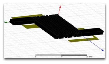
*Figure 5: Three-dimensional band-pass filter structure with DGS structure*
