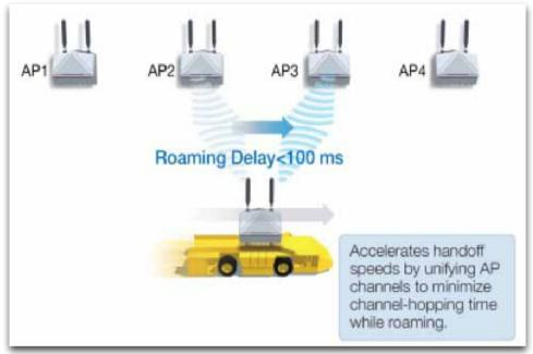
Figure 11: Example illustrating turbo roaming [source: 9]
