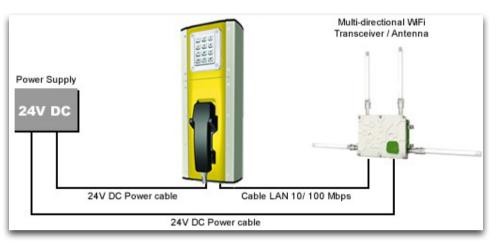
*Figure 2: A Wireless Emergency Telephone system [source: www.norphonic.com]*
