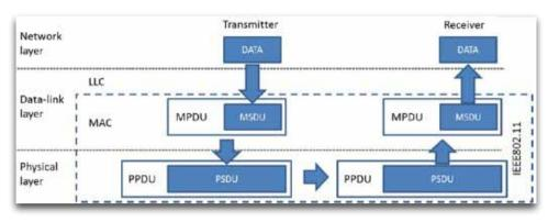
Figure 4: Simplified view of OSI model and packet encapsulation.
