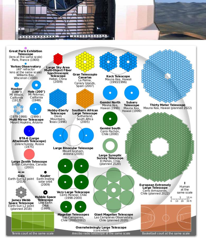
A comparison of the primary mirrors of the world's largest telescopes.
