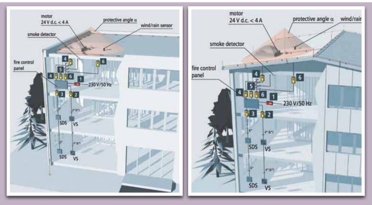
Figure 1: Domelight located in the protected volume of an air-termination rod on a non-metal roof of a structure with external lightning protection system.
