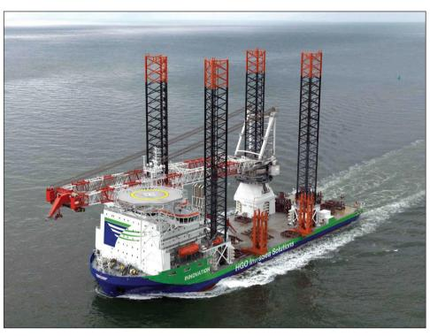
Ship Innovation – has a load capacity of 8,000 tons and can install in waters up to a 65 meter depth.
