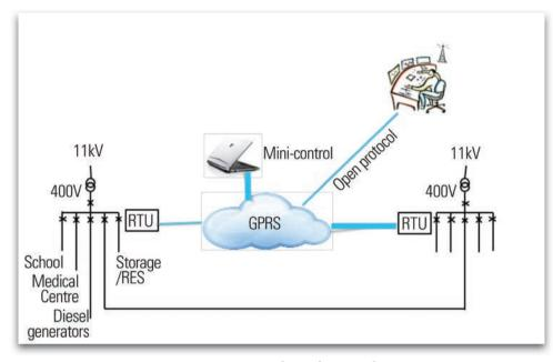
Figure 5: Microgrid interface to utility
