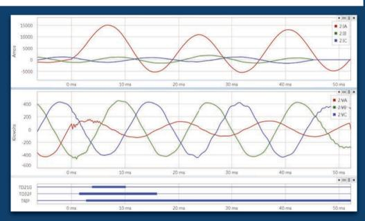
Shown here is the performance of the SEL-T400L for an phase A to ground fault on a 500 kV series-compensated line. The SEL-T400L issued a TRIP command to open the breaker in 2.8 ms; this is 6 times faster than present day phasor-based protective relays.
