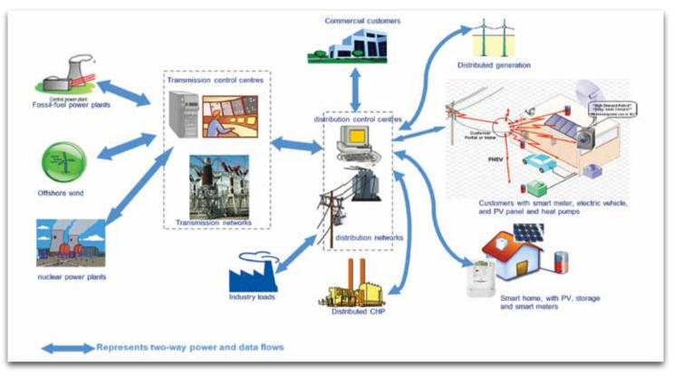
Figure 2: Smart Grid Example (Merz and McLellan)
