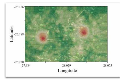
Figure 2 - Gaussian smoothed lightning density map based on SALDN data from 2007 - 2015. The Brixton and Hillbrow towers are indicated in the image and can be distinguished by the "hotspots".
