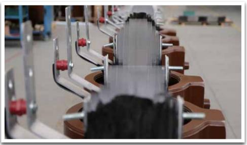
Fig. 5 - View of the lamination of the core.
