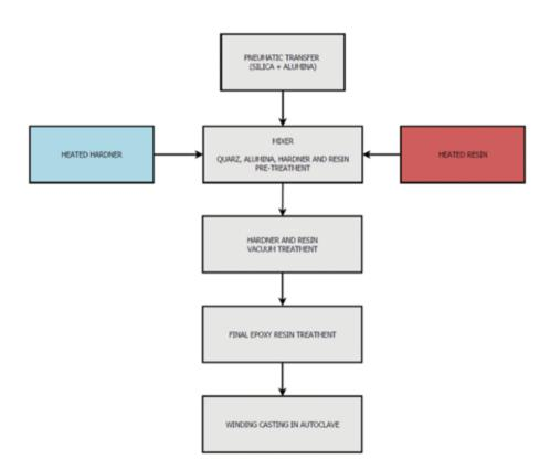
Fig. 8 - Casting system flow chart.
