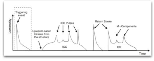
*Figure 5 - Luminosity against time for an upward lightning flash.*
