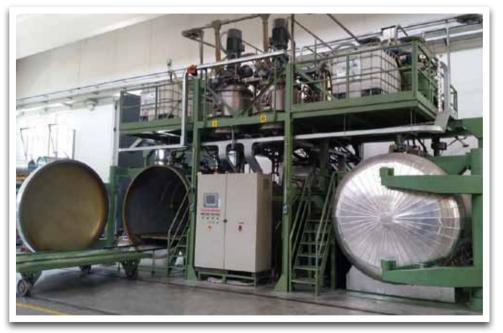
Fig. 9 - Autoclave for high voltage coils.
