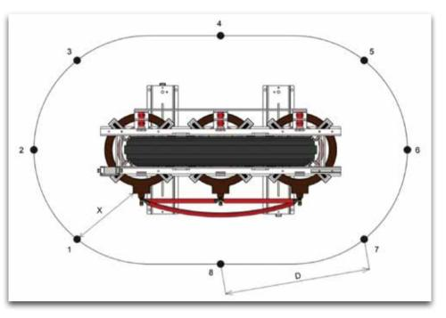
Fig. 16 - Microphone positions for point-by-point measurement.
