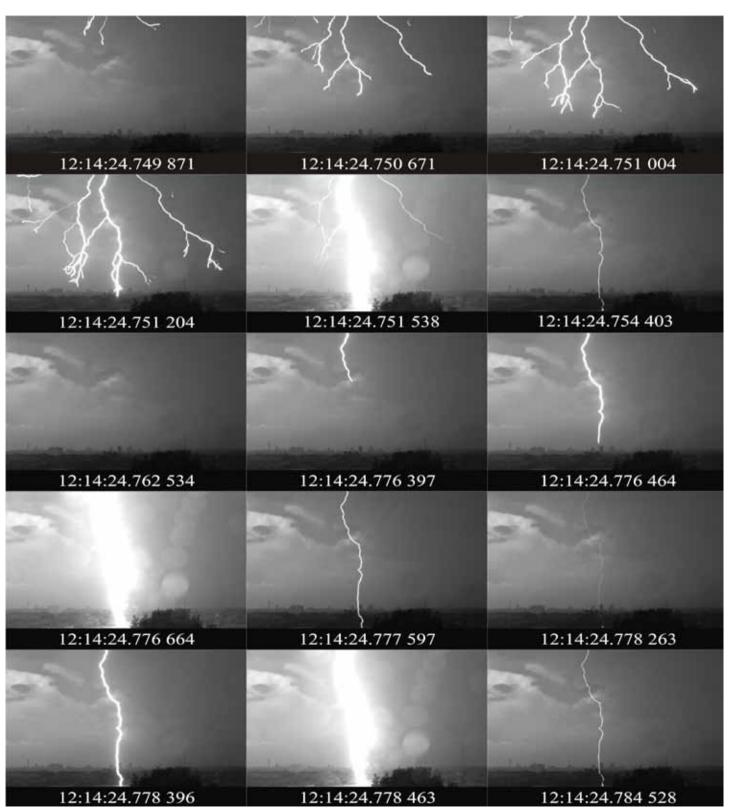
Figure 3 - High speed video frames of a negative downward flash over Johannesburg.
