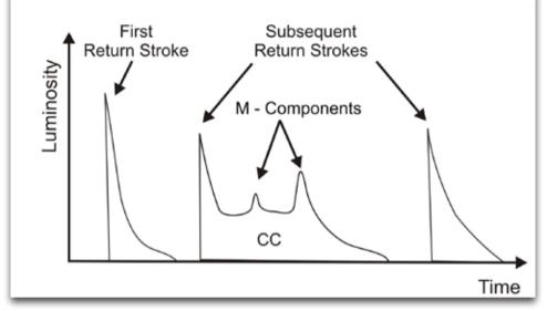
Figure 4 - Luminosity against time for a downward lightning flash.
