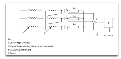
Fig. 18 - Basic measuring circuit for the partial discharge test for a three-phase transformer
