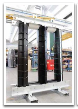
Fig. 10 - Magnetic core.
