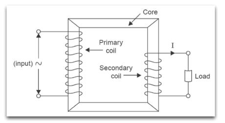
Fig. 1 - Primary coil is energized, secondary coil is loaded.
