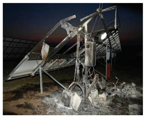
Damaged Solar Plant due to Lightning
