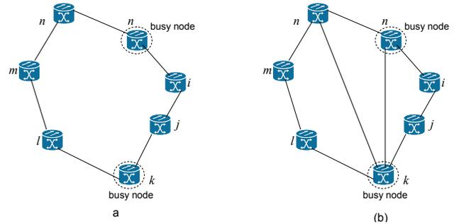
Figure 2. Networking topologies: (a) ring and (b) mesh [6].
