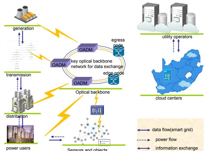
Figure 1. Smart Grid and support Network infrastructure.
