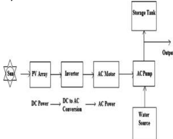
Figure 4: Direct coupled solar pumping system [18].
