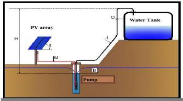
Figure 1: Basic Solar System for Boreholes [8]
