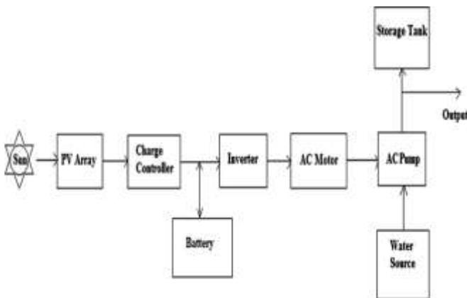
Figure 3: Battery coupled solar pumping system [18]
