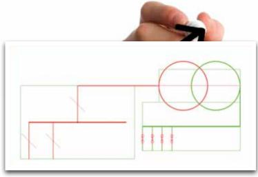
Figure 2: Minisubstation connected network model, allowing for 11kV cable connections to 11kV ring main unit (left), transformation from 11kV to 400V (upper right) and connection to LV cable circuits at LV fuses (right)
