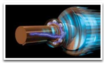
Damaging shaft voltages going through bearings on the way to earth.
