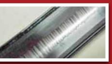
Damaged Grease & Bearing fluting, "washboard" pattern on bearing race
