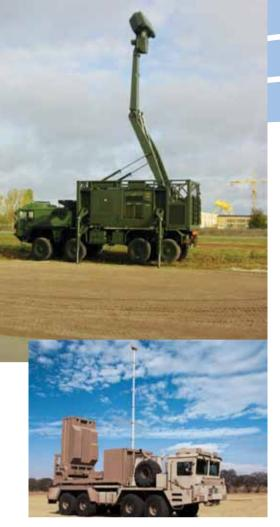
Typical Giraffe surveillance radar (top) suitable for the proposed ground-based air defence launcher system.
