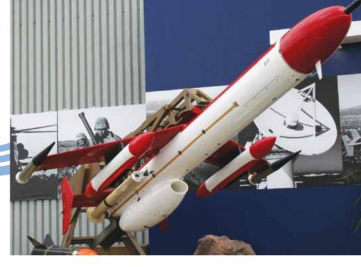
Skua, Denel Dynamic's high-speed target drone, is designed to simulate high-speed attack aircraft during land, sea and air combat training exercises and weapon development.
