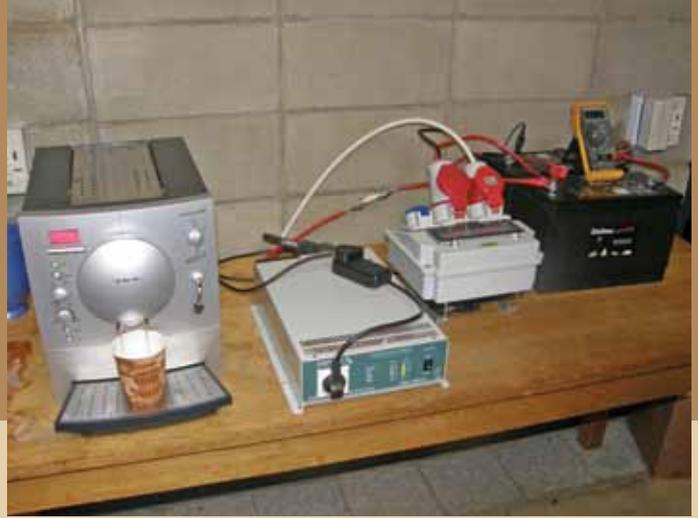
The wind powered coffee system – a cappuccino machine, inverter and a battery pack – being recharged by a wind turbine on the roof.
