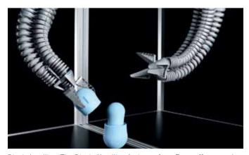
Bionic handling: The Bionic Handling Assistant from Festo offers complete flexibility and the ability to safely move objects from one position to another.
