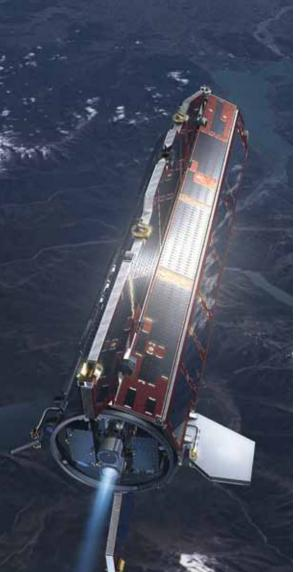
This artist's impression shows the GOCE satellife (Gravity Field and Steady-State Ocean Circulation Explorer), that will map the Earth's gravity field. It will orbit at a relatively small distance of 260 kilometres from the surface of the Earth. For this reason, GOCE has a sleek aerodynamic design and comes equipped with special ion thrusters. Credit: ESA.
