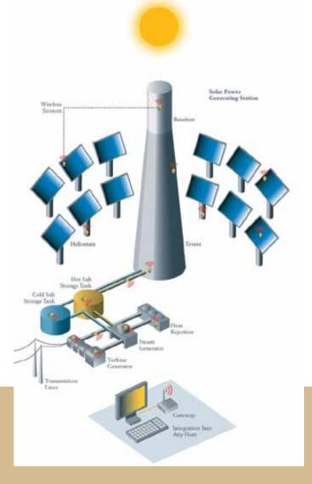
A diagram of a concentrated solar power plant. Mirrors are used to focus sunlight onto a single point at the top of a the tower.
