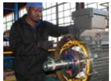
A B5 flange being fitted at the Zest WEG Group's Middelburg facility.
