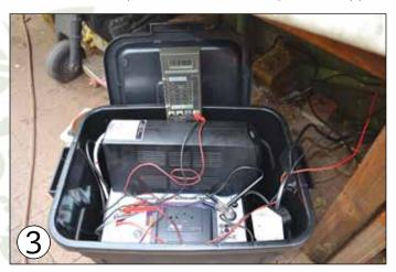
The Steca PWM 6,0 A charge controller sits between the solar panels and the 102 Ah Raylite SMF100 battery. The battery is in turn connected directly to the inverter, which is actually a 600 VA computer UPS.
