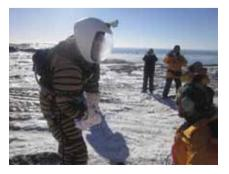
to Mars. The \$100 000 suit was designed by Argentine aerospace engineer Pablo de Leon and tested at Argentina's base in Antarctica.
