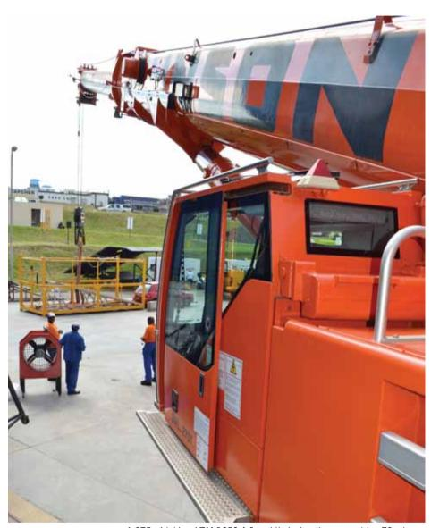
A 275 t Liebher LTM 1250-6.1 mobile hydraulic crane with a 72m boom was used to hoist the car in its cradle.
