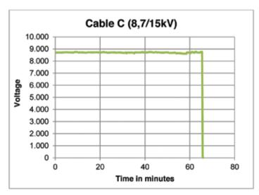
Figure 5: Test result and time breakdown.
