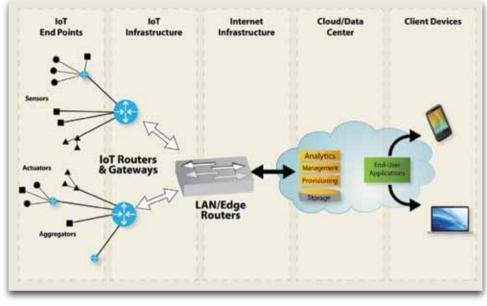
*Figure 1: IoT connectivity includes the traditional M2M connected devices, but extends across the network, to the cloud, and beyond.*
