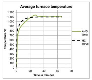
Figure 2: Average furnace Temperature
