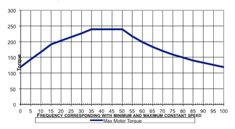
Thermal envelope for VSD driven electric motors
