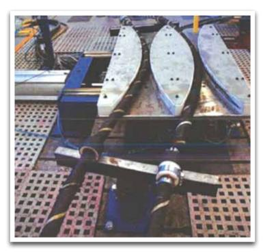
Figure 2: Bending against template test arrangement
