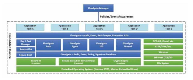
Figure 3: A complete security framework that leverages hardware security features.
