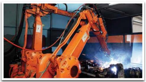
Two robots are used to load, unload and weld parts with little human intervention and with a high degree of accuracy
