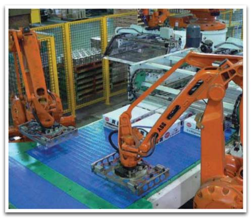
Robots elevate the nature of work by reducing large lifting requirements in this facility
