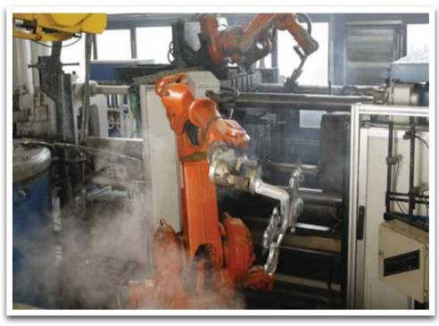
Two robots work in coordination to remove and deburr the part, then spray the die to prepare for the next drop. This application of robots also removes humans from this high temperature environment
