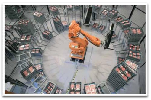
A single robot is used to organize small quantities of inventory to efficiently stage individual orders to be shipped
