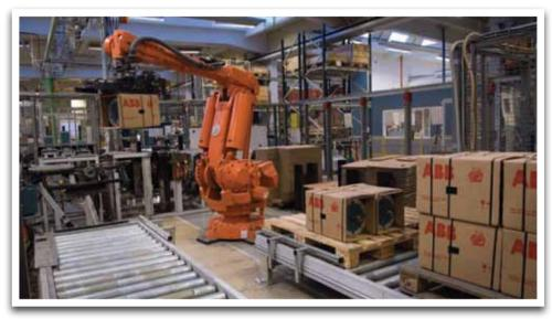
Robots speed the palletizing of motors while reducing waste, and the concern of a worker being hurt
