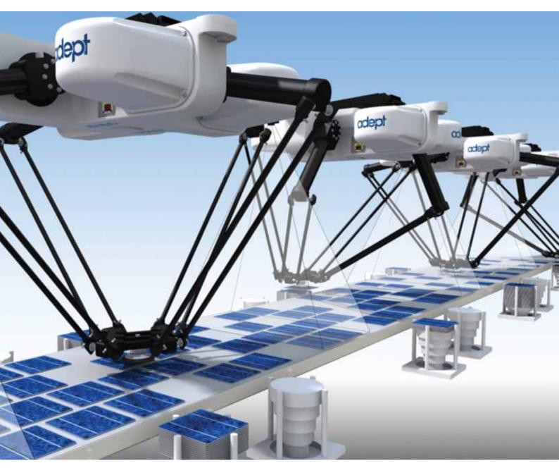
solar cells and even whole modules and then place the gripped objects with great precision and speed.
