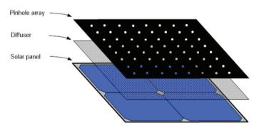
Figure 1: Absorber structure
