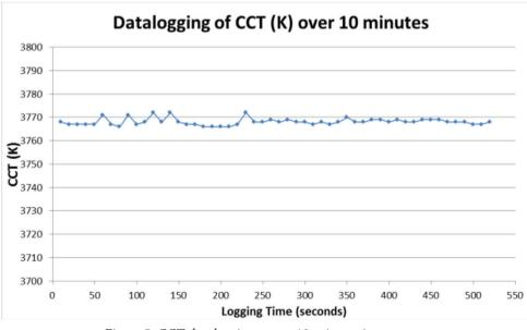
Figure 5. CCT datalogging over a 10-minute time span.
