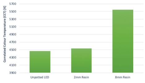
Graph 5 - Effect of resin thickness on colour temperature shift
