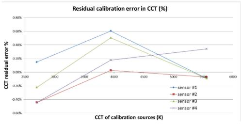
*Figure 4 presents the residual error in CCT for each sensor; it shows the residual error in CCT* (*K*) is  $\pm 0.6\%$  for the three tested CCTs of 2,700K, 4,000K and 5,600K.
