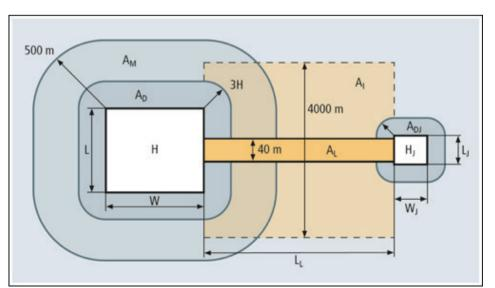
*Figure 1: Areas from which lightning strikes can cause damage to a building, its incoming lines and its systems*
