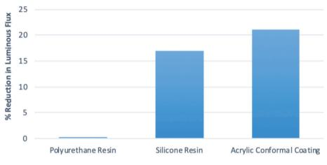
Graph 4 – Change in luminous flux after exposure to mixed corrosive gas
