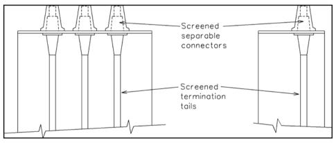
Figure 8: Screened separable connector termination – inside cone (type 5)
