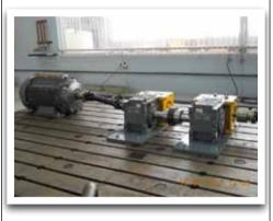
Specialist drive engineering company SEW-EURODRIVE offers customers the peace-of-mind that all of its gearboxes meet the necessary quality standards and requirements, thanks to the load test bed which is currently only found at the company's Durban branch.
