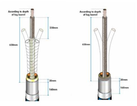
*Figure 10: Example of screened and belted PILC cable termination prepared from the top down principle*
