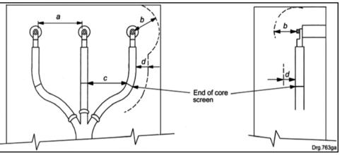
Figure 4: Bare termination Air-insulated (type 1)
