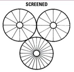
Figure 1: Unscreened (belted) cable and Screened cable PILC MV power cable
