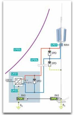
Figure 2: When setting up a mobile network transmission station with remote radio head technology, the division into multiple lightning protection zones has become even more important.
