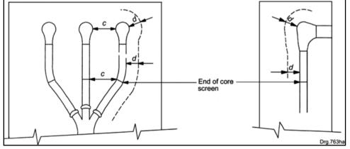
*Figure 5: Shrouded termination (type 2)*
