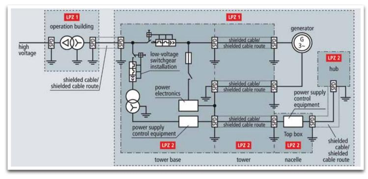
Figure 5: Example of arresters installed at the zone boundaries of a wind turbine according to IEC 61400-24
