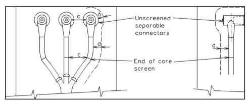
Figure 6: Unscreened separable connector termination (type 3)
