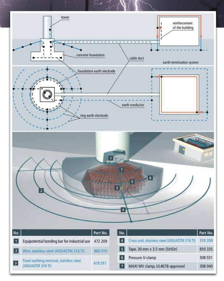
Figure 3 - Earth-termination system of a wind turbine
