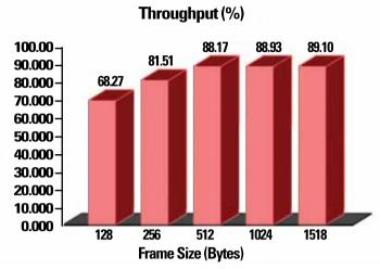
*Figure 1: Results of an RFC 2544 throughput test. Each frame size is measured individually.*
