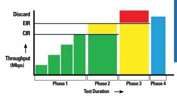
*Figure 2: The four phases of the* Y.1564 *Configuration Test. The duration of each phase is user defined.*
