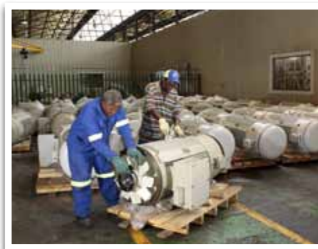
Two members of ACTOM Electrical Machines' factory staff are seen here doing finishing touches to one among a large batch of 250 kW squirrel cage induction motors awaiting delivery to SPX for installation in air-cooled condensers for Kusile power station.
