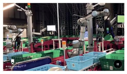
Figure 7: Robots at a Japanese's Factory picking items from bins to assemble order[19]
