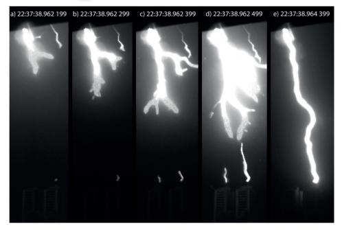
Figure 1: A sequence of frames from one of the high-speed captures of a lightning attachment to the apartment building on the left.
