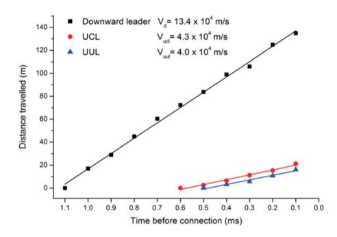
Figure 2: Distance versus time plot and linear regression fits for the downward leader and the upward connecting leader (UCL) and upward unconnecting leader (UUL). The gradient of the linear fits gives an indication of the average speed of propagation [2].
