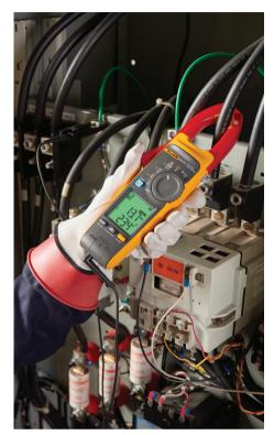
The Fluke 377 FC and 378 FC True-rms clamp meters use Field-Sense™ technology to make testing faster and safer, all without touching a live conductor for accurate voltage and current measurements.
