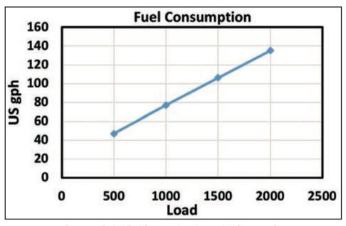
Figure 9 – Typical Fuel Consumption of a 2000kW Generator Set
