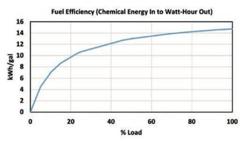
Figure 10 – Typical Diesel Generator Set Fuel Efficiency
