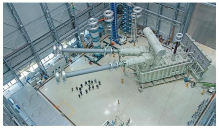
1,1 MV 587,1 MVA Siemens single phase 800-ton converter transformer
