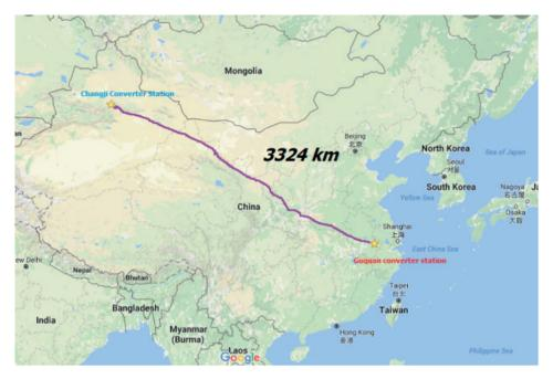
The 1,1 MV 12 GW UHV DC Changji-Guquan power line was completed in 2019. This 3324 km line has set new world records in terms of voltage level, transmission capacity and distance.
