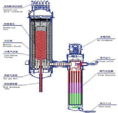
Figure 2: The PBMR HTGR Design Layout
